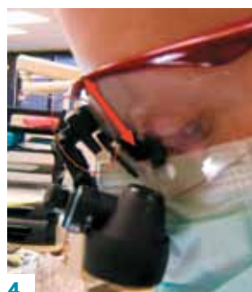
4 ▲ A vertical slide feature ensures that the scope sits low enough in relation to the pupil to maximize declination angle.
